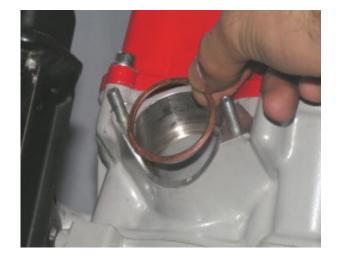
Put the primary tube gasket into the primary tube port.
