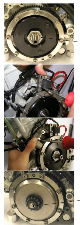
Install the clutch onto the crankshaft (do not forget the key).
