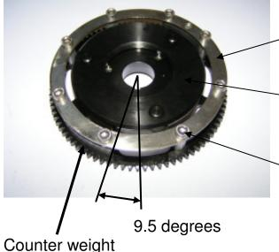
Tighten the unit with 3 bolts M7 and 3 bolts M8 by applying a torque of 22Nm.
