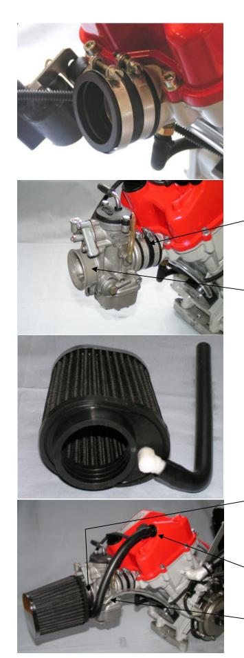
Put the two hose clamps onto the carburetor rubber and push the rubber onto the intake port.
