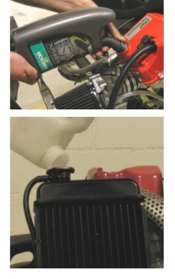
Fill in 0.4I 0W30 motor oil from "Motorex" into the engine.
