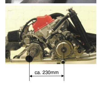
Now install the engine onto the gokart. The distance from the middle of the rear axle to the middle of the crankshaft is 230mm.
