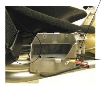
Remove the battery and the rubber floor.
