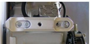
The bolts of the engine mount have to be tightened with Loctite 243 and 22Nm torque.
