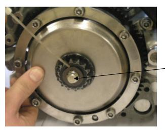
Push the clutch drum backwards and apply chain spray between transmission sprocket and thrust washer.
